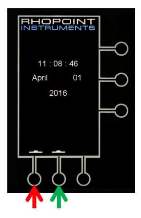
Press the button marked with a green arrow to start adjusting the time and date.
