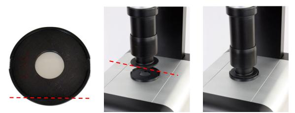
Take a reading on the checking standard by pressing the tick icon and compare the result with its assigned value. The value must match the assigned value within the tolerances printed on the label.
