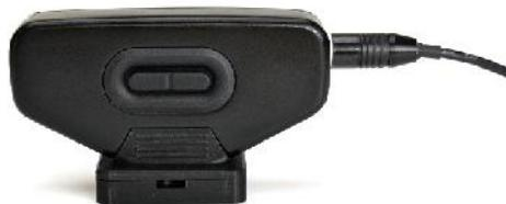
Place the measurement head and calibration holder on a flat surface and initiate calibration.
