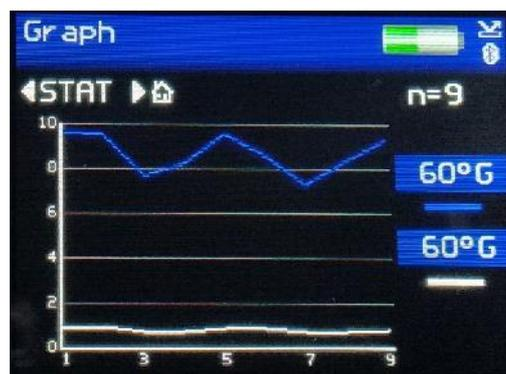
When pressing the up / down buttons NG data can be displayed either all together or individually.
