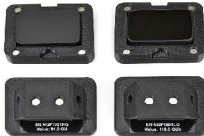
The calibration tiles are enclosed in a magnetically sealed holder.
