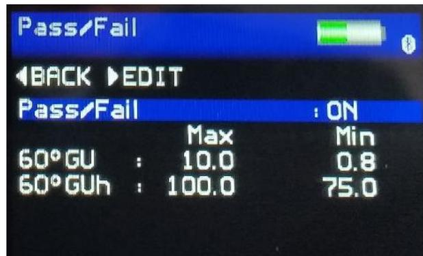
The Pass/Fail setup screen is used to enable/disable on-screen pass/fail indication and set min / max tolerances.
